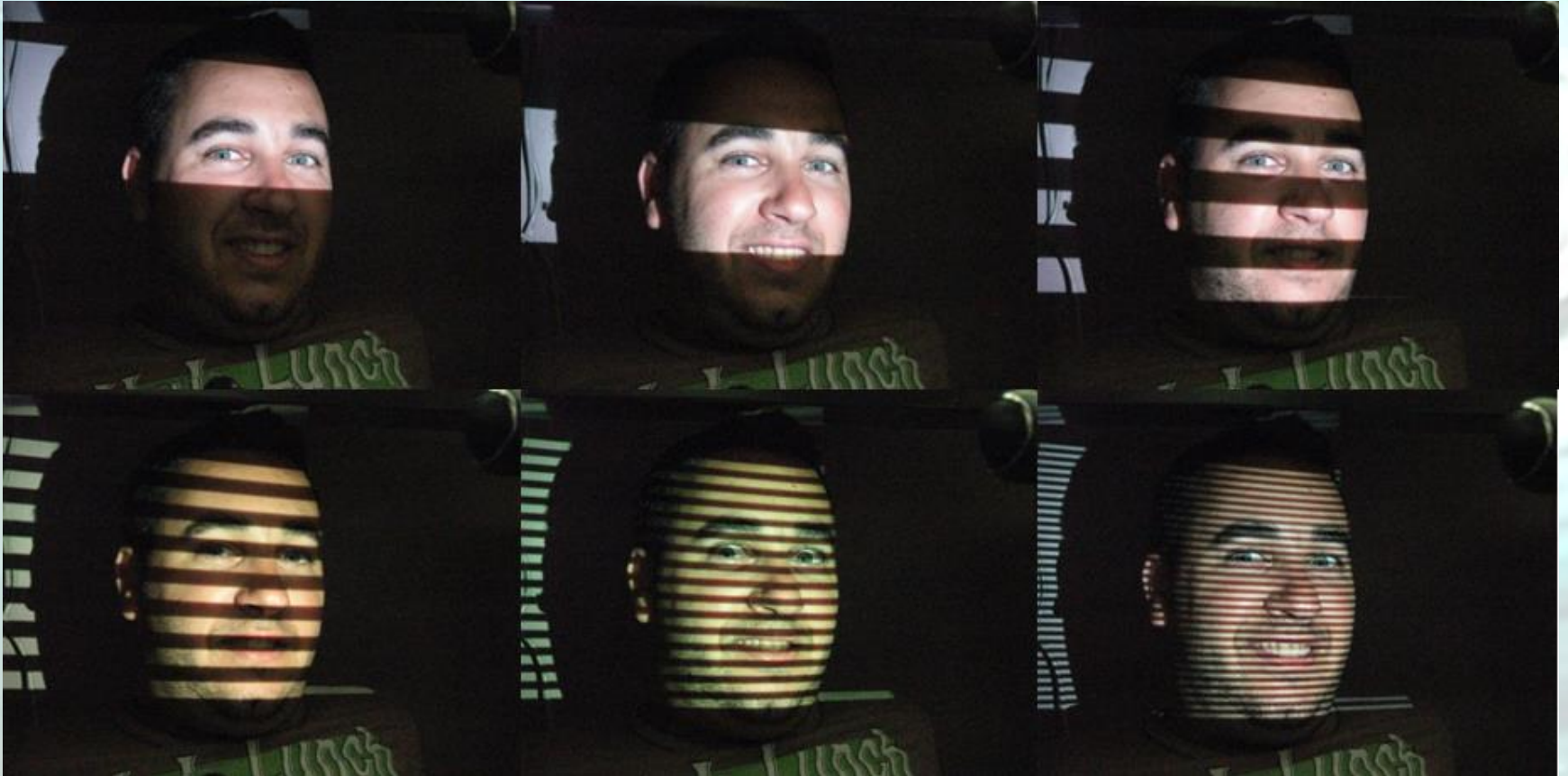
Figure 14 – Coded light projected by the pico projector
